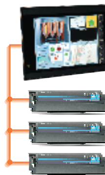
Industrial Computer/CE-based Controller with SmartStix Fieldbus I/O on DeviceNet or PROFIBUS network
