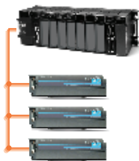
Programmable Controller (PLC) with SmartStix Fieldbus I/O on DeviceNet or PROFIBUS network
