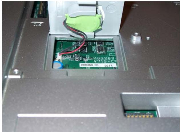
Figure 13.2 – Battery Compartment
