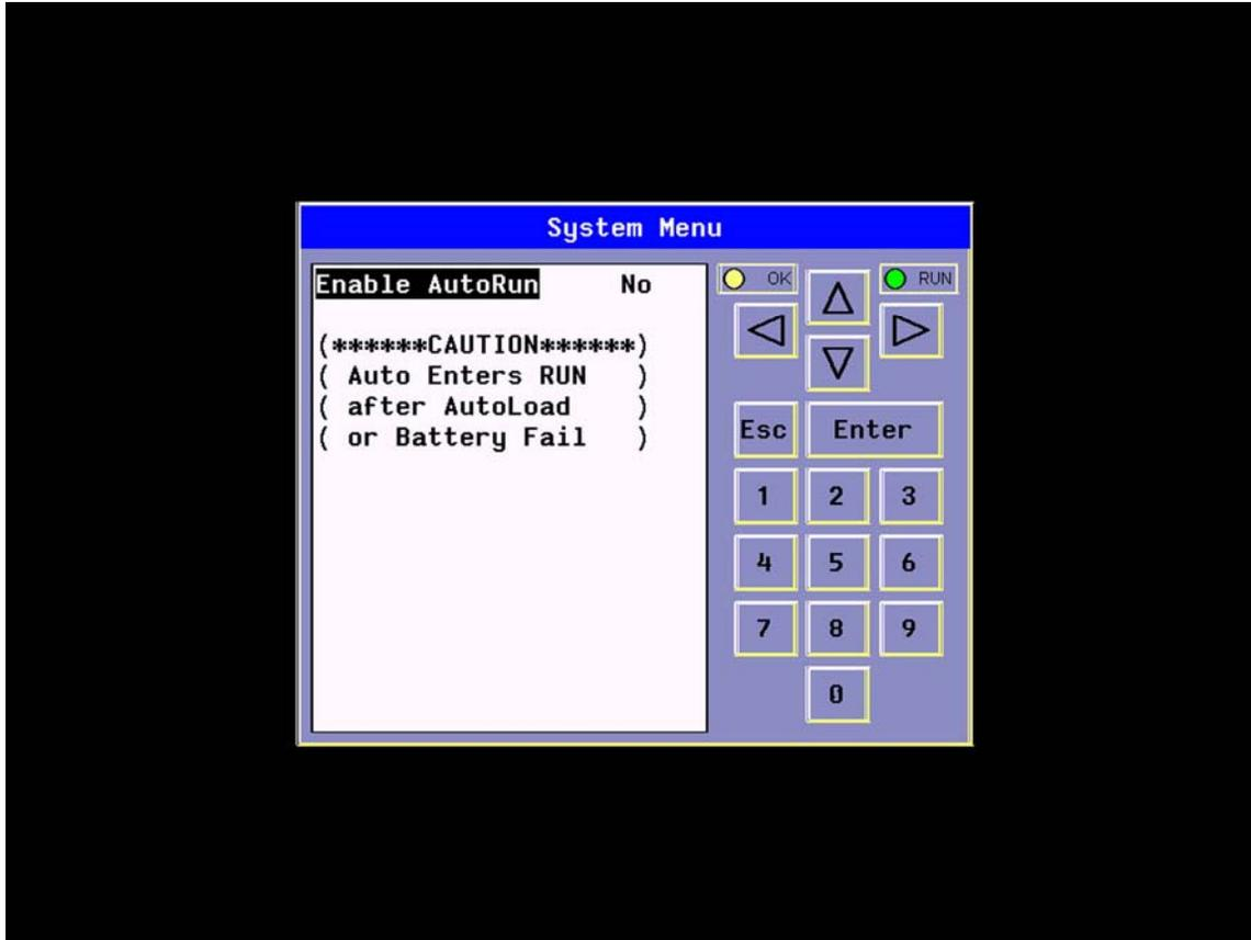
Figure 14.12 – Enable AutoRun Yes/No System Menu
