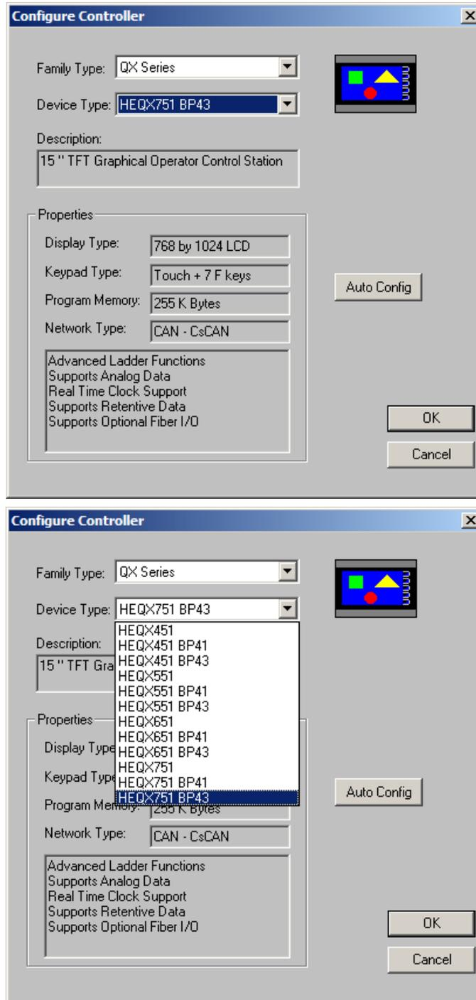
**Figure 7.2 – Configure Controller Screen**
