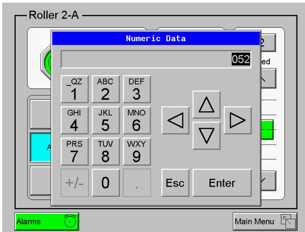
**Figure 10.2 – Alpha-numeric Keypad**
