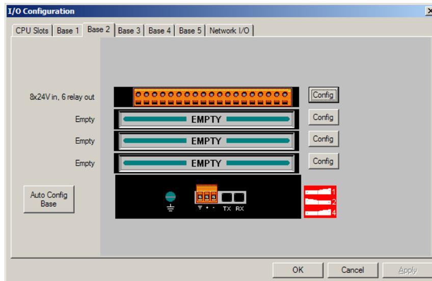
Figure 7.6 – Base 2 with an I/O Module Selected
