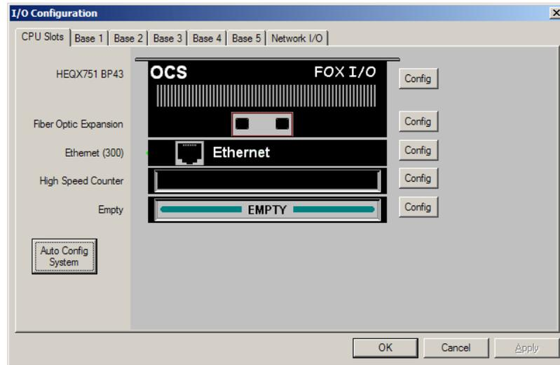
**Figure 7.3 – Main Base Screen appears with QX751 and BP43**
