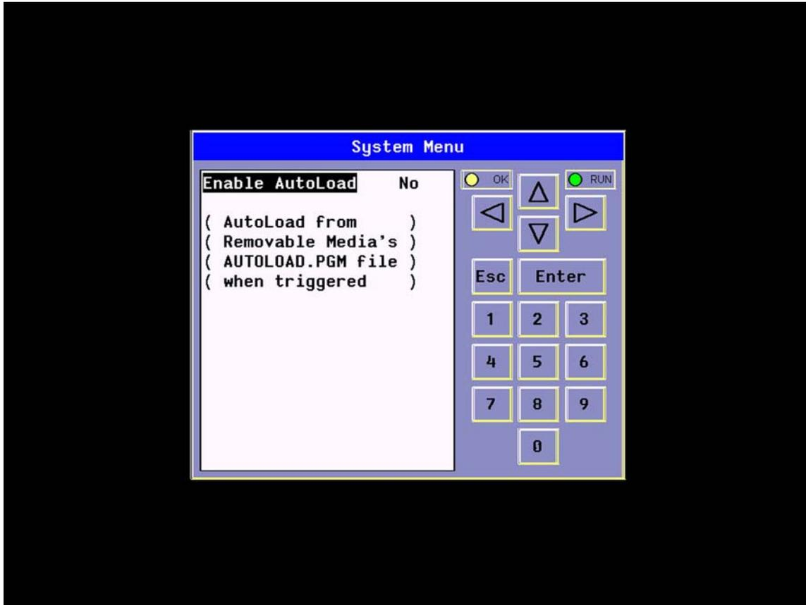
Figure 14.9 – Enable AutoLoad Yes/No System Menu
