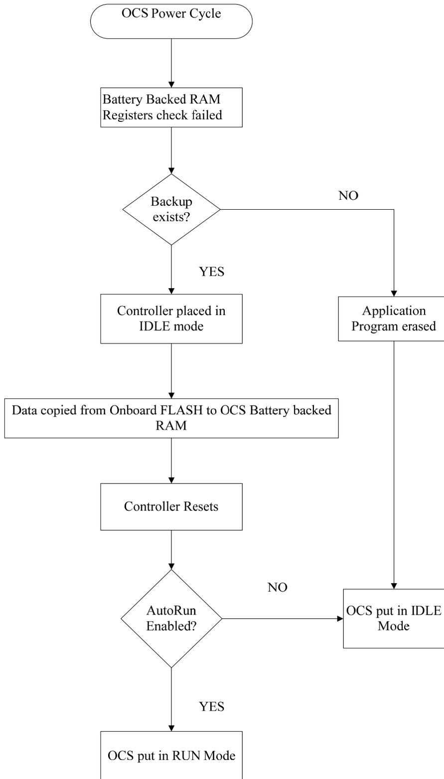
Figure 14.7 - OCS Sequence in Execution of Auto Restore
