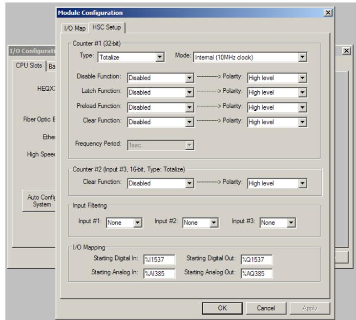
Figure 8.5 – Built-In HSC Configuration Screen
