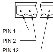
Figure 8.1 – I/O Port (HSC/PWM) Terminal Connector
